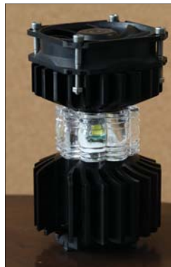
250W Led light source for Metal Halide Lamp replacement
