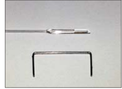
OCT Endoscopic Probe (Diameter: 0.25–2mm)
