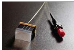
NIR scanning grating spectrometer with size of only 2.3 cm 3
