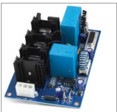
IGBT controller board for partial discharge flashlamp pumped Lasers
