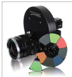
First ever multispectral imaging instrument extending sensitivity through UV wavelengths
