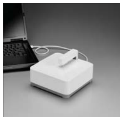
aRTie measures spectral R, T, R+T, A(=1-R-T), and color of flat specular samples
