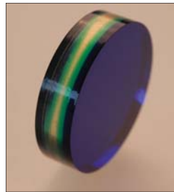
Absorbing filter stacks are durable, cleanable & exhibit no angle shift
