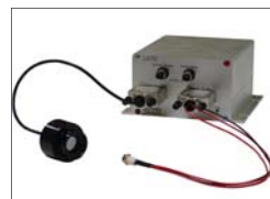
LIV110. Laser diode characterization: powerful, low cost LIV test system
